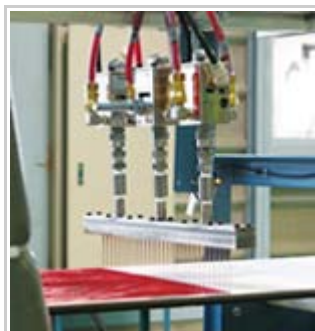
⑥ 補強材裏貼
